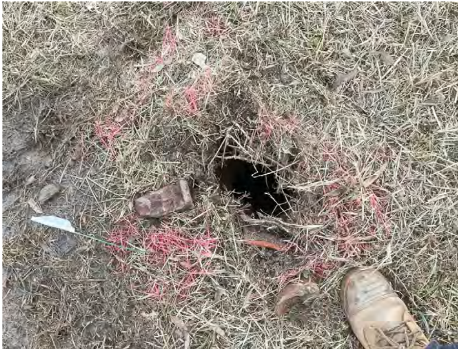
Photo 7 - Brick structure and void encountered whilst drilling BH05
