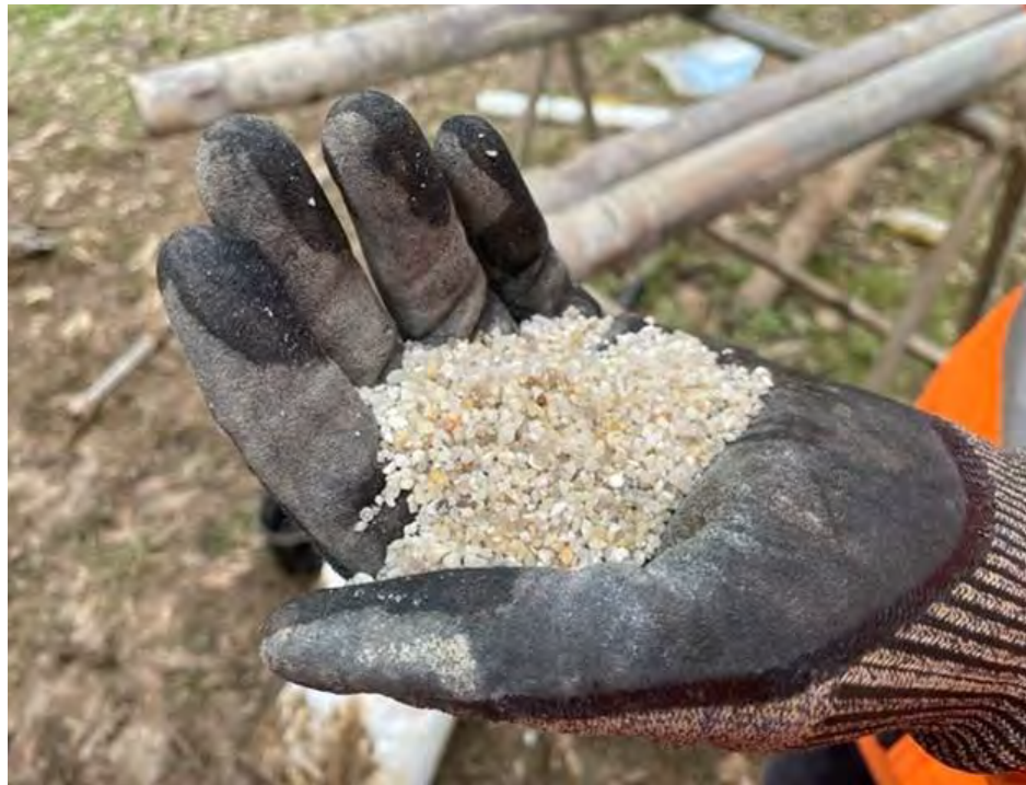
Photo 10 - Specialised Sand' material used for gravel pack/filter pack in piezometers
