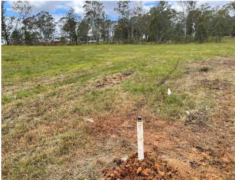
Photo 9 - Completed standpipe piezometer (BH09)
